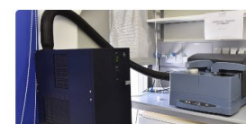
M-DSC (Modulated Scanning Calorimetry)
